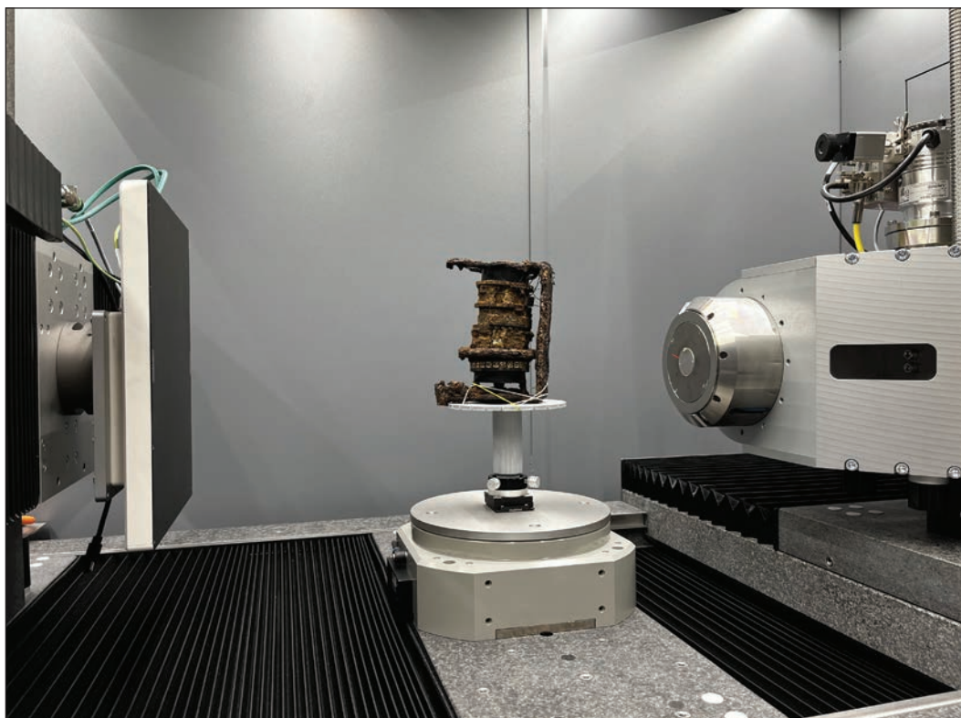
Figure 3: Enigma M4 rotor block on a stand, placed in an EasyTom XL Ultra microCT device (Photo: Miha Hren).
