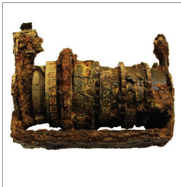
Figure 2: Enigma M4 from the minesweeper R 15; wheel compartment during conservation (Photo: Andrej Gaspari).
