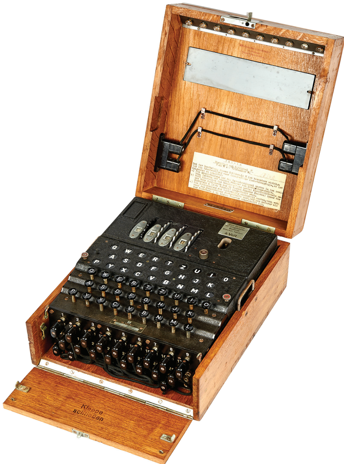
Figure 12: Enigma M4 electromechanical cipher machine was developed primarily for the U-Boot division of the German Kriegsmarine. The machine was housed in an oak carrying case (Source: Cryptomuseum, 2022).
