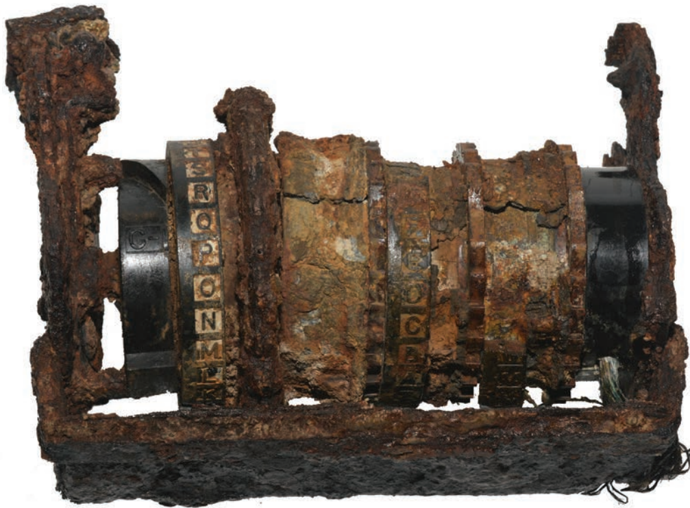
Figure 9: Enigma M4 from the minesweeper R 15; wheel compartment after conservation (Photo: A. Gaspari).
