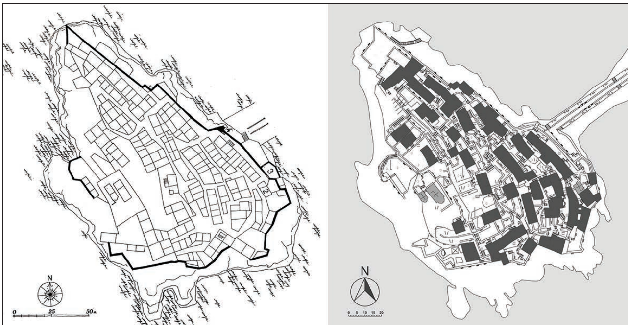
Figure 3: The structure of the settlement of Sveti Stefan before adaptation (left) and after adaptation (right) (Source: Mijović & Kovačević, 1975, 134; Cadastral map of the Budva Municipality (segment from drawing)).
