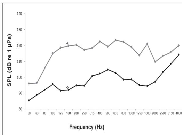
**Fig. 3:** 1/3 octave band Sound Pressure Level spectra (*x*-axis in logarithmic scale, 10 Hz – 4 kHz) of the noise produced by a passenger cruise liner under normal operational conditions (line with diamonds) compared to the local background noise level (line with dots) (sampling frequency 44.1 kHz). The frequency in which the passenger cruise causes the maximum increase in the background SPL level is depicted with stars.
