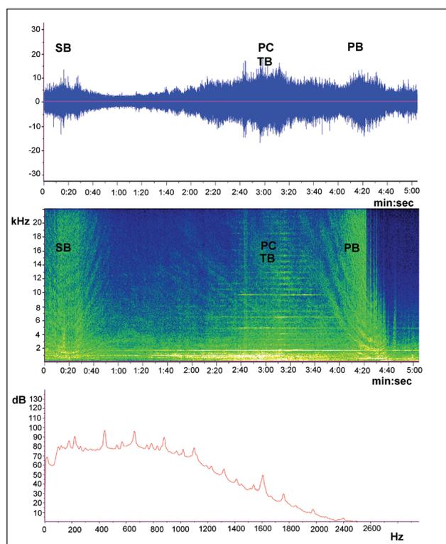
**Fig. 2: Oscillogram (top), spectrogram (centre) and power spectrum (bottom) of the noise emitted from a passenger cruise liner crossing the Lido tidal inlet. A five second time period has been chosen for calculating the noise spectra (from 2:45 to 2:50 of the recording). Filter bandwidth 10 Hz, sampling frequency 44.1 KHz, 50% overlap, window Blackman Harris. SB - speed boat, PC - passenger cruise, TB - tug boat, PB - pilot boat.**
